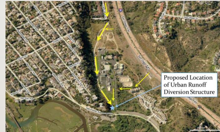
This project aims to capture the stormwater (urban runoff) around the San Elijo water reclamation facility area by a collection system and then pump this collected water to the existing treatment plant to produce really clean recycled water.
